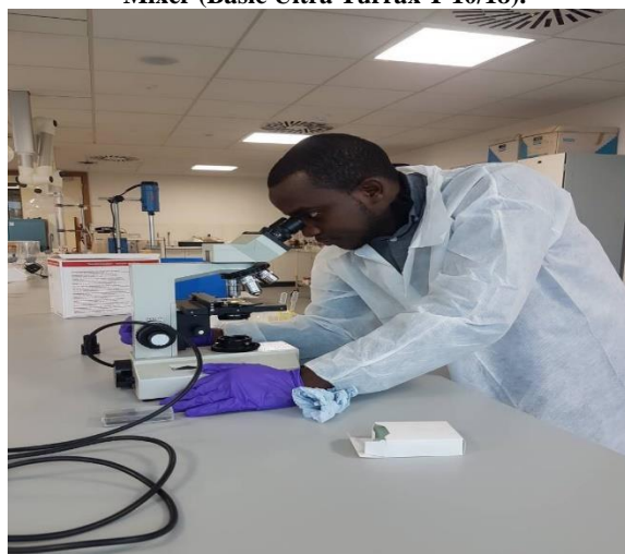
Figure 2: Microscopic Droplet Size Analysis Using A High Precision Light Microscope (Olympus CX 31)
