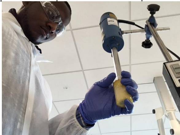
Figure 1: Dispersion of Oil in Water Using High Shear Mixer (Basic Ultra Turrax T 10/18).
