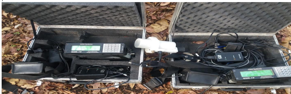
Figure 3: GEM's GSM-19 Overhauser Magnetometer Equipment.
