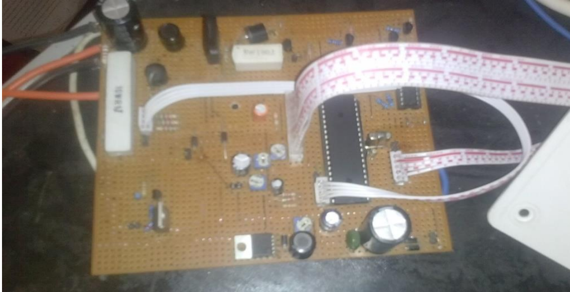
Plate 1: The final construction of the charge controller
