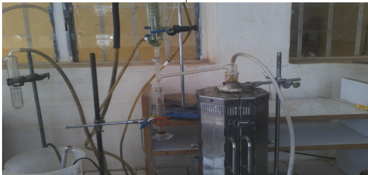
Plate 1: Reactor Set-up for Pyrolysis Process
