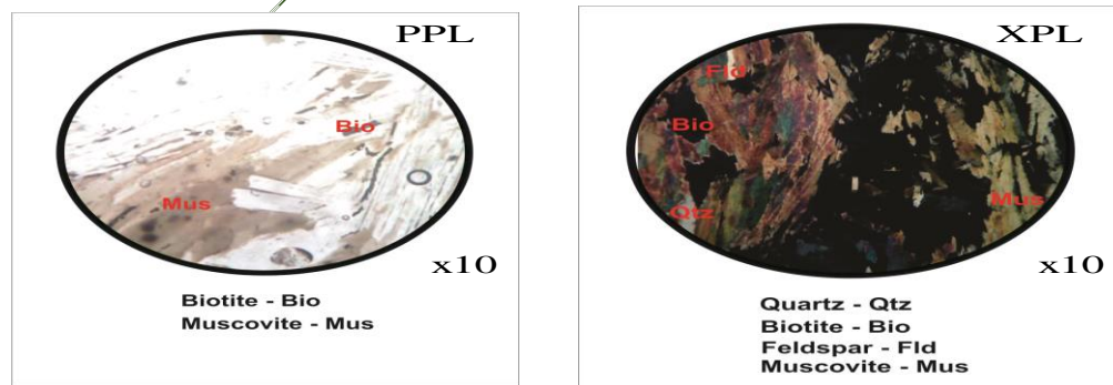
Figure 7: Photomicrograph of rock sample from L4 at Jiko under PPL and XPL (Magnification = x10).
